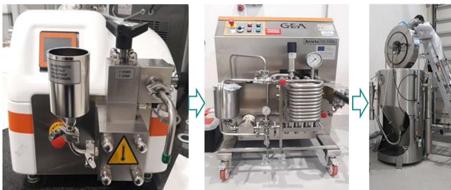
Fig.1. Change of scale for the production of nanomaterials: from 6L/h to 100 L/h.
